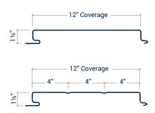
Flat-12 & Flat-12R are a concealed fastener soffit/liner panel. It is available in 24 gauge only.
