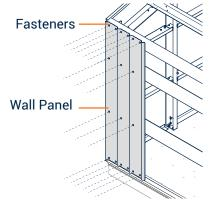
Install Top & Bottom fastener line first before securing middle of panel.
