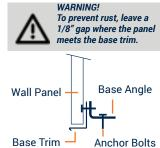
Concrete foundation and anchor bolts not provided by Whirlwind.
