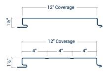
Flat-12 & Flat-12R are a concealed fastener soffit/liner panel. It is available in 24 gauge only.
